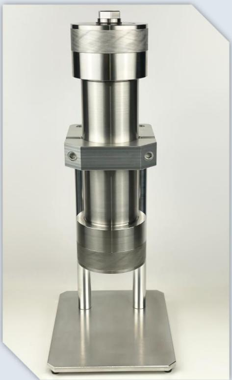
Floating Piston Accumulators (Transfer cylinders) are used in oil and gas/chemical industries to store and displace liquid and gases for laboratory experiments.
